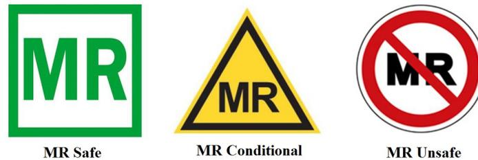
**Figure 5.3:** The standardized icons MR Safe, MR Conditional, and MR Unsafe as defined in ASTM F2503 [240]
