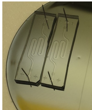
Figure 3.12. Fabricated PDMS serpentine chamber still bonded on the valves mold.
