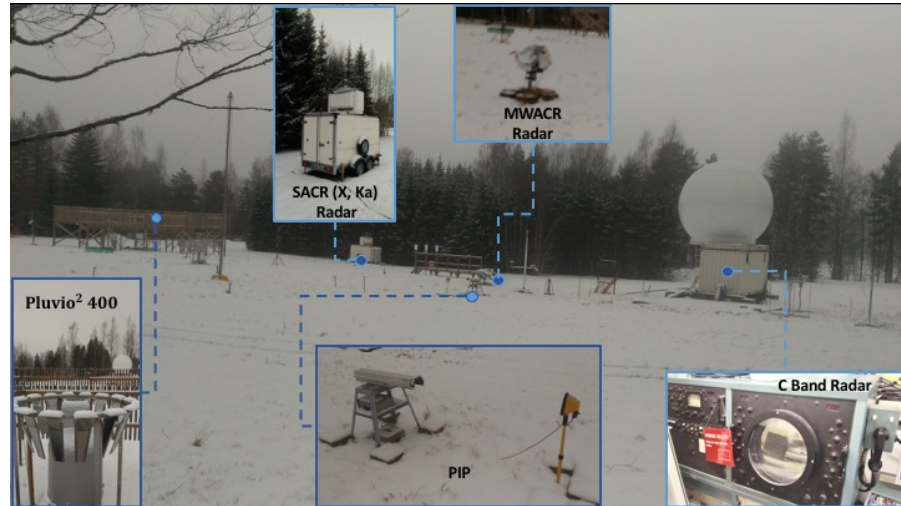
Figure 62: Measurement site shown with in situ and remote sensing instruments during the BAECC campaign 2014 at Hyytiälä, Finland.
