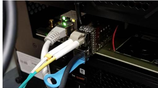
Figure 5.4: The SFP+ connectors provided by the Trenz Board.
