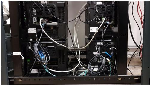
Figure 5.3: The ExaNet development platform shaping  $2 \times 2$  topology.
