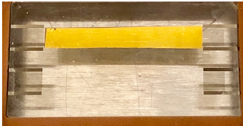
4.6 The delay line on ST-cut Quartz substrat
